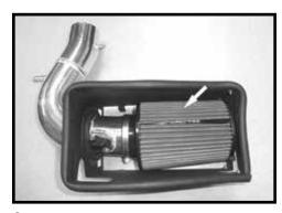
Step 7 Install the filter onto the intake tube.
